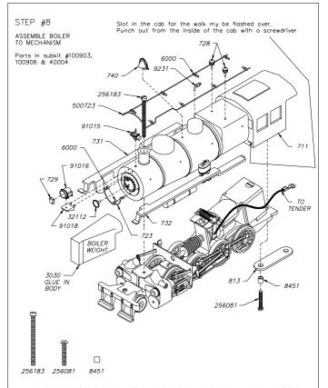
DO NOT PAINT BOILER UNTIL AFTER THOROUGHLY TEST RUNNING THE COMPLETE MECHANISM.
