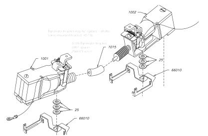
The T-1 Duplex require 22" radius curves. To make the T-1 work on 18" RADIUS follow the following steps.
